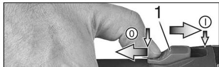
**Switching on/continuous operation:** Push the slide switch (1) forward. For continuous operation, tilt it downwards until it engages.
